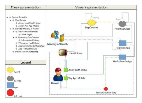
Figure 7: Architecture of cross-device tests with mobile and Digital-TV
