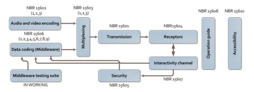
Figure 1: Technical standards for the digital TV ISDB-T standard [ABNT 2004]
