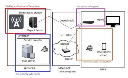
Figure 8: Instance example of the proposed metamodel
