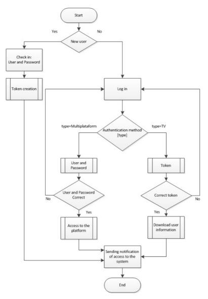
Figure 5: Basic authentication process proposed for architecture
